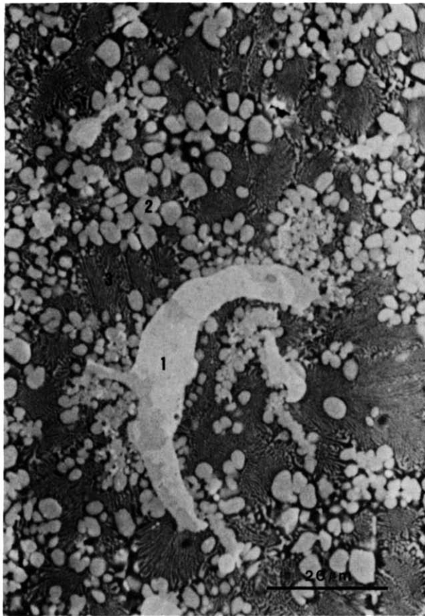
Fig. 5. SEM micrograph showing a globular morphology of the ZrO_2 phase observed in sample 01. Again, marks 1, 2 and 3 are representative of the predominantly metallic region, ZrO_2 dendrites and Al_2O_3 - ZrO_2 eutectic, respectively.
